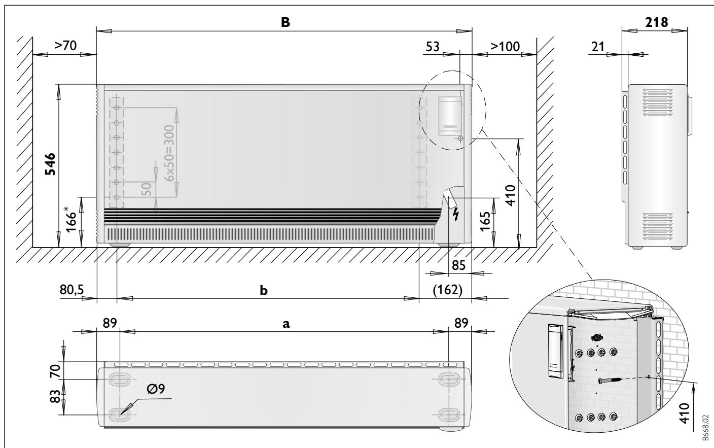
\* Installation with floor clearance possible, see Pos. 2.4.2 "Floor-free Heater Installation with wall fixing brackets"
