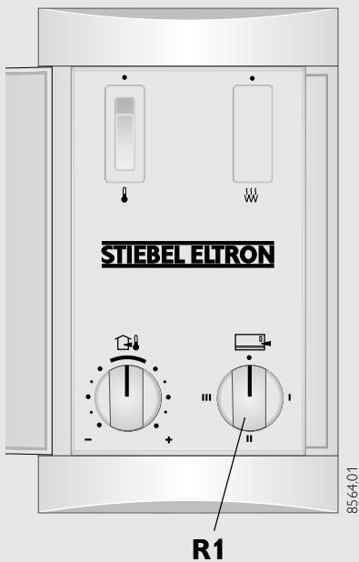
**Heat storage** (charging) – infinitely adjustable selector switch
